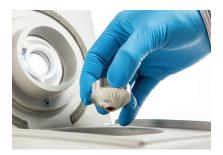
Figure 1. The ability of the Airfuge ultracentrifuge to spin small samples at high g-forces makes it ideal for clarifying lipemic samples. Powered by ordinary laboratory air pressure, the ultracentrifuge accelerates to speed in just 60 seconds. Tiny air jets levitate and accelerate the rotor. Turbine flutes machined on the bottom of the rotor provide the driving surface for the air jets.
