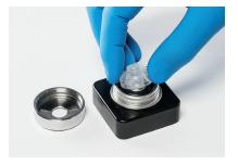
Figure 3. The base of the rotor is designed to completely support both chambers of the liner during centrifugation.
